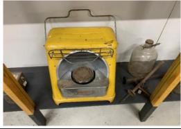
Left: This is an old "Fyrside" brand kerosene room heater. The glass bottle on the right had a valve in the cap so it could be inverted into the reservoir which is behind the burner. The burner had a strip of woven asbestos as the wick.
