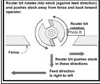
If the wood is introduced from left to right in the same direction as the bit is rotating the bit cutter edges instantly become very efficient high-speed power feeders that can suddenly eject the wood, leaving your empty hands dangerously close to the cutter.
