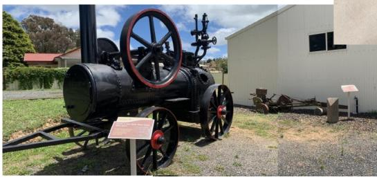
Left: This is a typical wood burning steam engine used on many farms for mechanical power before internal combustion engines became common.
