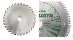
teeth are evenly spread around the circumference of the blade with an alternated tooth bevel (ie. the teeth lean in alternating directions). Further, the gullets on the crosscut blade tend to be somewhat shallow. The reason for the large number of teeth and the narrow gullets is because of the structure of cross grain which creates small chips. A cleaner cut is achieved by increasing the tooth count (which also increases the speed of the cut, with the short
