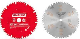
So, what does all this mean to you? For one, you should check what blade is installed before you go an make your cut. For example, the person before you may have been making a whole series of ripping cuts and had installed a ripping blade that may be unsuitable for your purpose if you wish to cross-cut. BE AWARE THAT COSS CUTTING WITH A RIPPING BLADE MAY GIVE YOU A RAGGED CUT!!
